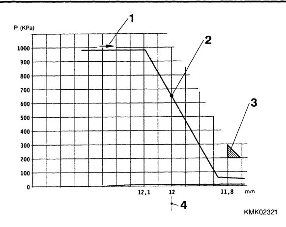
CHECKING SWITCHING POINT (EGR VACUUM CONTROL VALVE)
